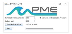
The miniDOT Plot program plots the files recorded by the miniDOT Clear Logger. The program reads all the miniDOT Clear Logger files in a folder, except the CAT.txt file. The program will also compute air saturation from the dissolved oxygen measurements. To do this, the program must know the air pressure and salinity. It calculates air pressure based on elevation of the water surface above sea level or uses the
