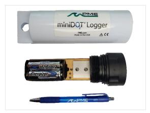
Caution: Do NOT remove the stainless screws in the black end cap. If this is done, then the miniDOT Logger will be permanently damaged and must be returned for repair.
