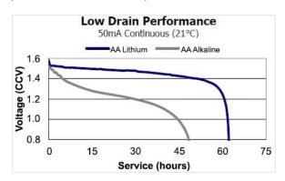
The figure below gives a general idea of terminal voltage vs. lifetime. Service life in hours is incorrect since miniDOT Logger draws far less than 50 mA continuously, but the general shape of the voltage vs. time gives an estimate of life remaining. This plot is taken from the manufacturer's specification. The plot is for a single battery. Double the voltages shown to give the terminal voltage as measured in the picture above. The miniDOT Logger halts operation at a total of 2.4 Volts.
