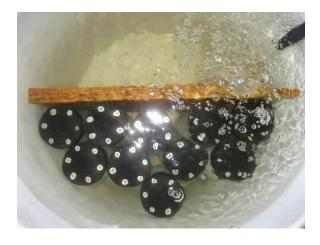
Record measurements for several hours or a day, but in any event long enough for the miniDOT Logger's temperature to come to equilibrium with the water. During the experiment, find the local air pressure, either from measurements or from a local weather station. Watch out... weather stations often report barometric pressure referenced to sea level. You must determine the absolute barometric pressure at your elevation.
