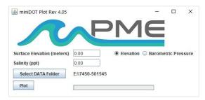
The miniDOTPlot program plots the files recorded by the miniDOT Logger. The program reads all the miniDOT Logger files in a folder, except the CAT.txt file. The program will also compute air saturation from the dissolved oxygen measurements. To do this, the program must know the air pressure and salinity. It calculates air pressure based on elevation of the water surface above sea level or uses the barometric
