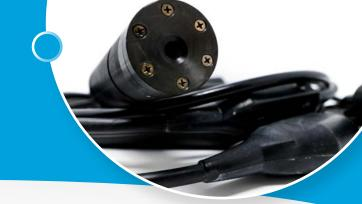
The T-Chain is a waterproof electrical cable containing a range of integrated water quality sensors for vertical profiling. Every T-Chain is constructed on a semi-custom basis, with users specifying the length, interval, type and quantity of pre-constructed sensors included. The central electrical cable is manufactured specifically for PME, featuring a Kevlar reinforced core and waterproof polyurethane sheathing.
