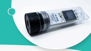
The fully submersible miniDOT® Clear Logger records dissolved oxygen (DO) and temperature measurements in fresh and saltwater environments. Its oxygen-sensing optode utilizes a fluorescence method to determine concentrations of dissolved oxygen in mg/L. Sampling anywhere from once per minute to once per hour, the miniDOT® Clear Logger's clear plastic housing contains an LCD display of DO and temperature in real-time. Data is recorded to the logger's internal SD card.
