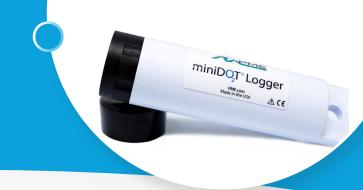
The fully submersible miniDOT® Logger records dissolved oxygen (DO) and temperature measurements in fresh and saltwater environments. Its oxygen-sensing optode utilizes a fluorescence method to determine concentrations of dissolved oxygen in mg/L. Sampling anywhere from once per minute to once per hour, all data is recorded to the logger's internal SD card.
