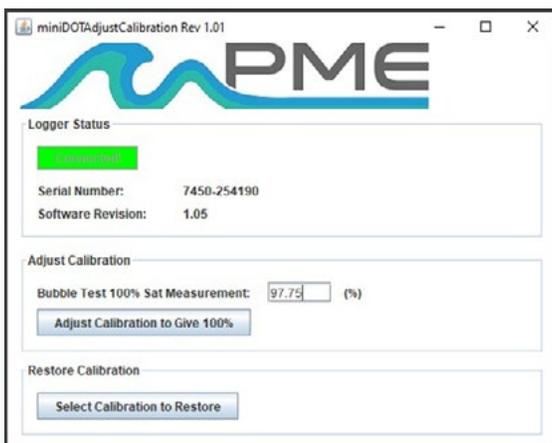
Adjustment of miniDOT® Clear calibration is accomplished by running the [miniDOTAdjustCalibration.jar](#) program shown below. Ensure the miniDOT® Clear being adjusted is connected to the computer running the adjustment program.
