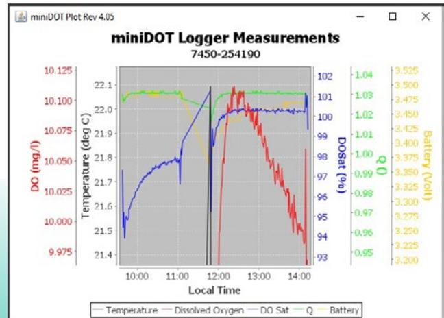
The above plot shows the first and second calibration verification experiments and highlights the improvement in accuracy post adjustment.
