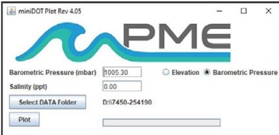
Upon completion of the experiment, plot the miniDOT® Clear measurements using **miniDOTPlot**, inputting the average measured barometric pressure during the experiment. Do not use elevation to approximate pressure.
