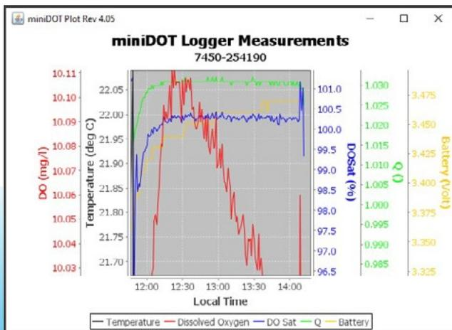
The plot above shows the results of a verification experiment that was performed immediately after the adjustment was made. It shows the saturation at only 0.5% higher than the expected 100%.
