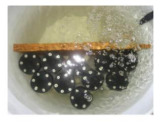
Record measurements for several hours or a day, but in any event long enough for the miniDOT Logger's temperature to come to equilibrium with the water. During the experiment, find the local air pressure, either from measurements or from a local weather station. Watch out... weather stations often report barometric pressure referenced to sea level. You must determine the absolute barometric pressure at your elevation.
